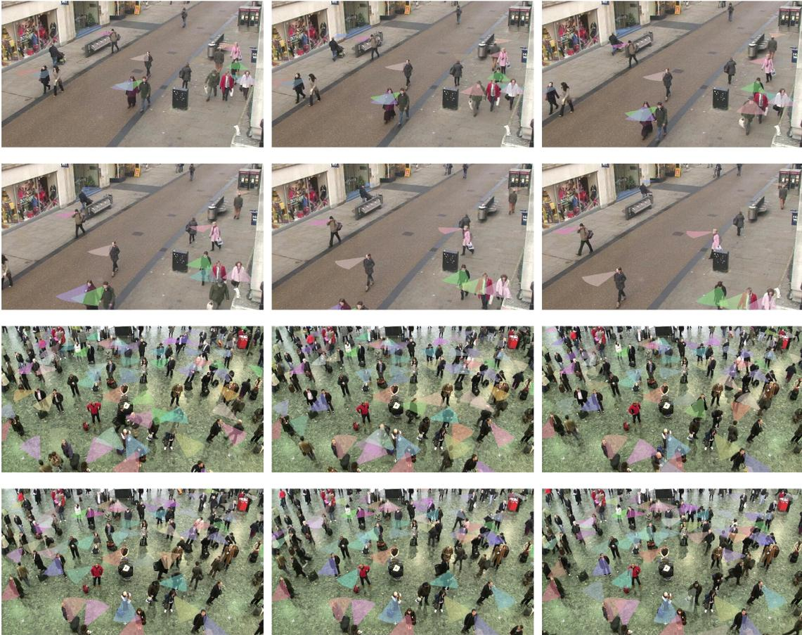
Figure 6.14: Frames from the two video datasets showing the estimated gaze directions drawn onto the people from which the automatic tracking extracted the head image sequences.
