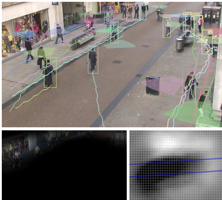
Figure 4: A frame showing the gaze direction estimates and the paths along which pedestrians were tracked. The lower images show the resulting attention map and the result of projecting it onto a video frame, identifying the shop window as a popular subject of attention. The blue lines on the attention map show the edges of the road.
